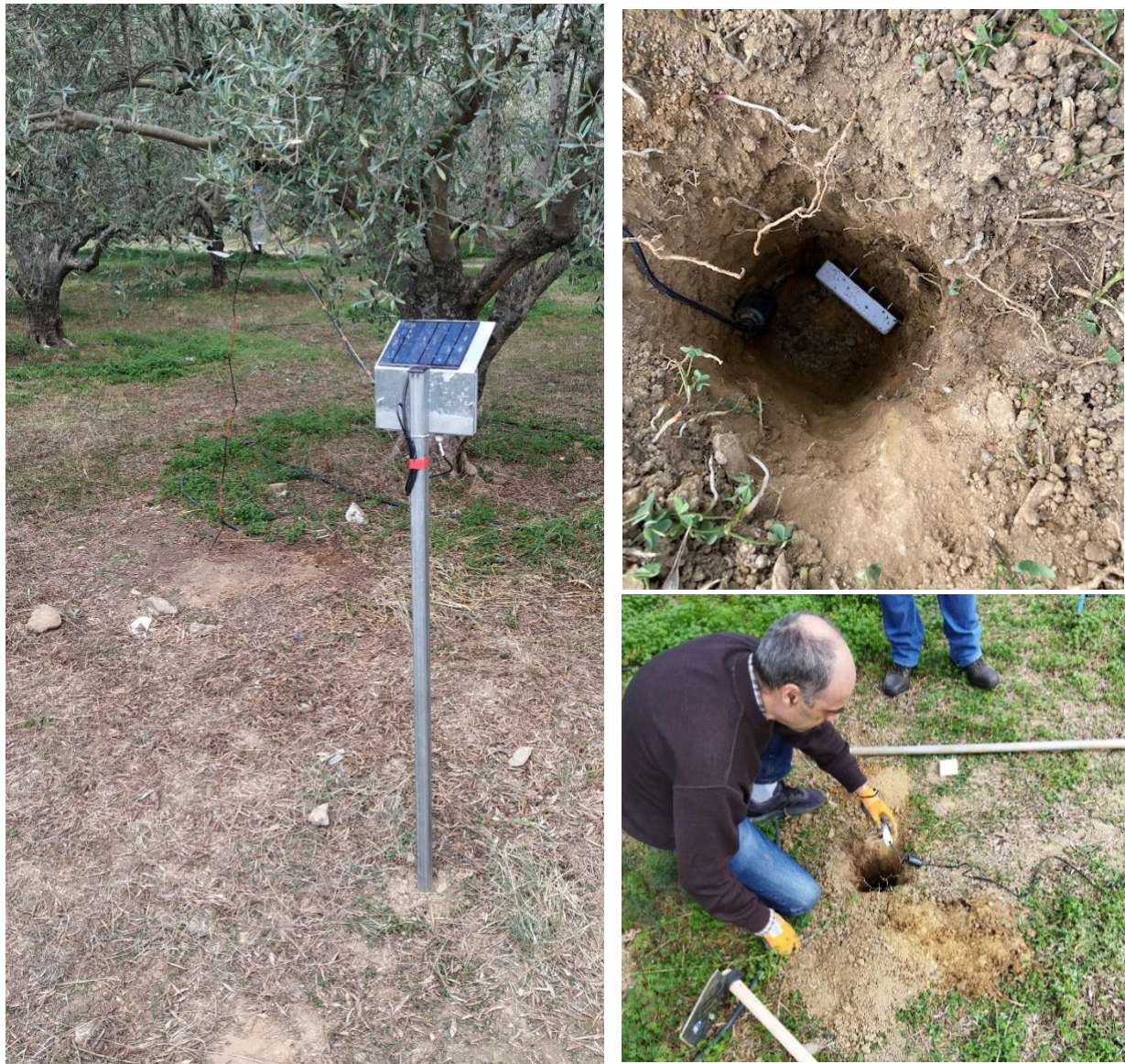
Figure 13. Installation of the soil moisture sensors as well as the whole telemetry soil moisture station.
