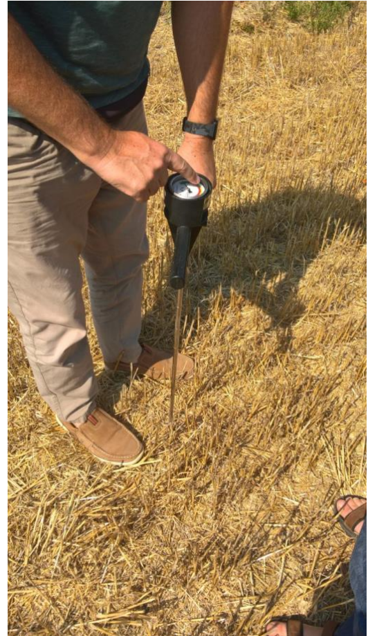
Figure 17. Checking the presence of plow pan on field using penetrometer after winter wheat harvest on a farm used in the use case in Serbia.
