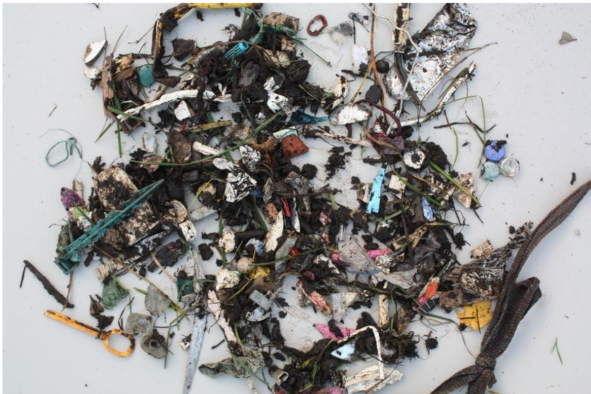
Figure 44. Contaminants removed by walk-over included: plastics, glass, ceramics, ferrous and non-ferrous metals, stainless steel etc.
