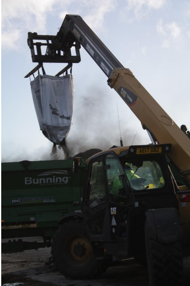
Figure 48. Bulk bags created safe-handling and dust issues during loading.
