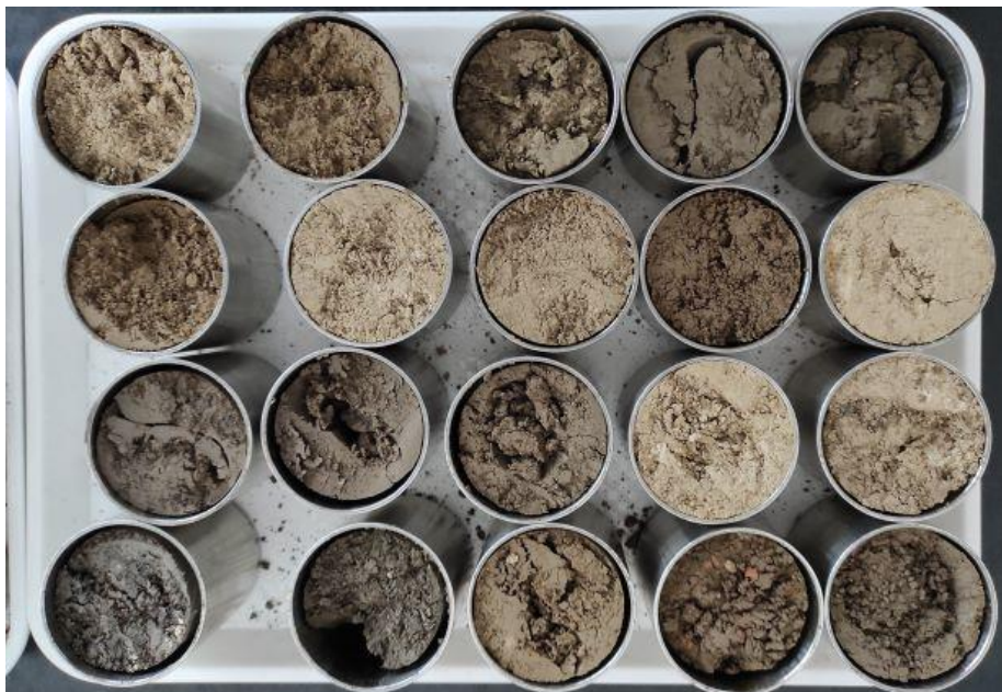
Figure 57. Soil samples in cylinders from different locations, soil types and depth after drying
